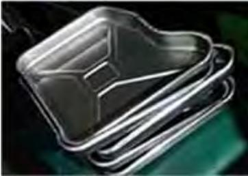
The flat sides of the can was stamped with a deep, large X-shape to stop the sides from bulging. The bottom corners were well rounded to minimise damage, the can was narrow so that it did not bump the legs when being carried, was tall enough to not require excessive stooping to pick it up and was rectangular in plane view to make them stack side-by-side efficiently.
